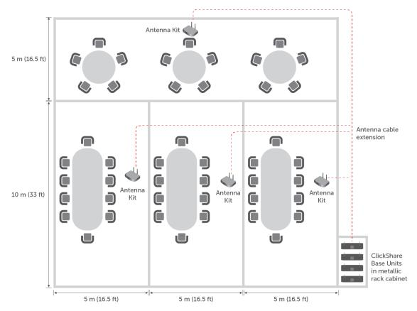
Figure: Example installation of antenna extension cables
