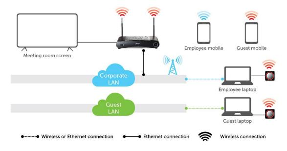
Figure: Out-of-the-box mode network topology diagram
