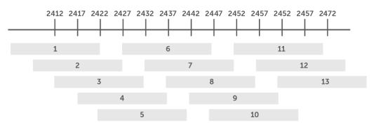
Figure: Wi-Fi channels in the 2.4GHz band
