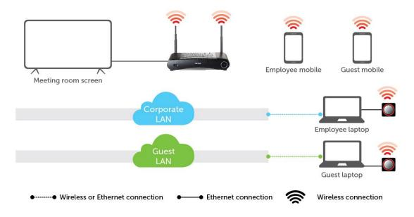
Figure: Out-of-the-box mode network topology diagram
